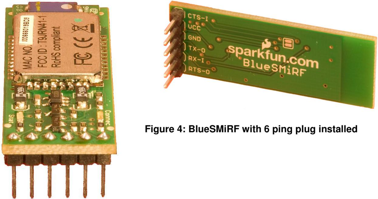
**Figure 4: BlueSMiRF with 6 pin plug installed**
