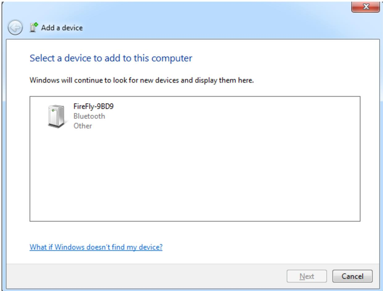
2) Windows will now search for active Bluetooth Devices. You should now Power up the LocoBuffer-Blue. It should find the LocoBuffer-Blue as a FireFly device as show above. The last few digits in the name are part of the Bluetooth address and will be different for each module. Select the FireFly icon and press the "Next" button.
