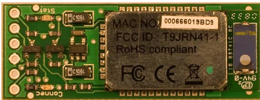
**Figure 1: Sparkfun BlueSMiRF Gold Module**
