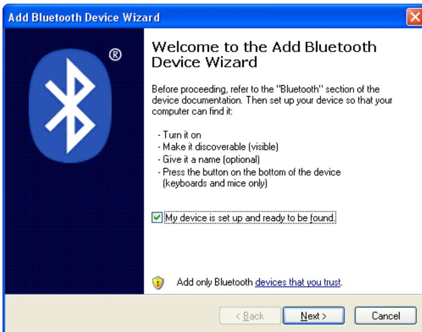
3) The Add Bluetooth Device Wizard should appear. Power up the LocoBuffer-USB, the Red led on the BlueSMiRF should be flashing. Check “My device is ready” and press **Next >**.
