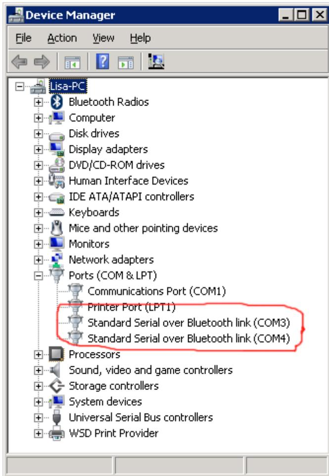
6) Go to the Start Button -> Control Panel -> Hardware and Sound -> Device Manager. The device manager window should now appear. Expand the Ports (COM & LPT) list. There should now be two “Standard Serial over Bluetooth link (COM\*)” devices. The lower numbered port (COM3 in the image above) will be the outbound connection port. You will use it to communicate with the LocoBuffer-Blue.
